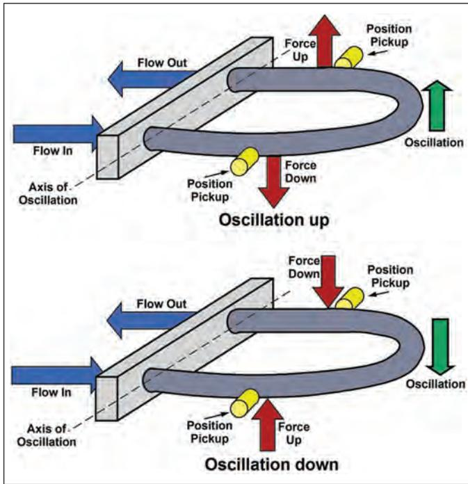
Figure 12: Principle of Operation for Coriolis Flowmeters
