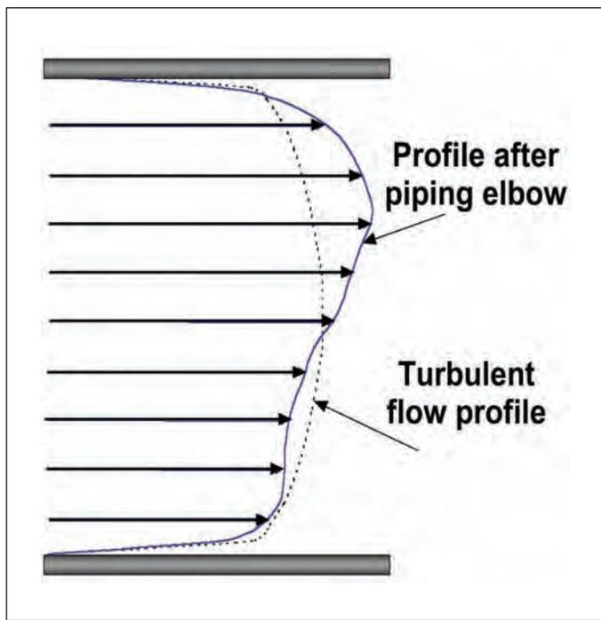
**Figure 2: Pipe Fittings Near the Flowmeter can Distort the Flow Profile, Requiring Straightening Devices.**
