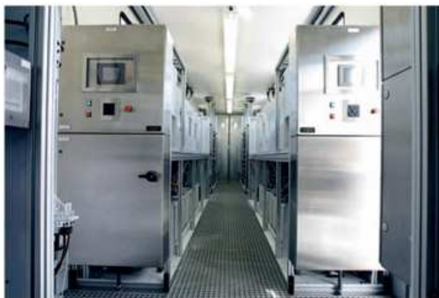
Figure 2: The Pilot Plant Contains Two Treatment Trains—One Mimics Full-Scale Plant and the Other is for Tests
