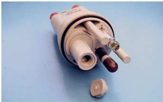
Figure 5: An Inexpensive, Replaceable Reference Junction Overcomes Problems of Blockages at Very Low Cost Two of the Eight New ABB pH 7653 Monitors Installed in the Pilot Plant
