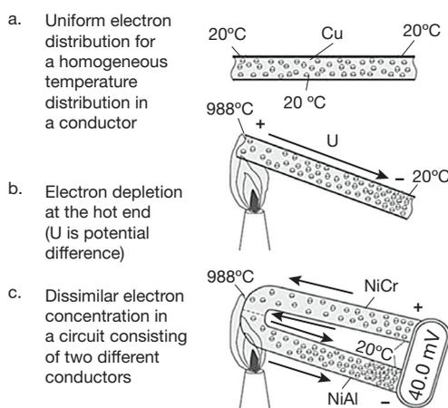
▲ **Figure 1.** As electrons accumulate at the cold end of a dissimilar-metal circuit, a voltage develops in proportion to the difference in the temperatures of the hot and cold ends.
