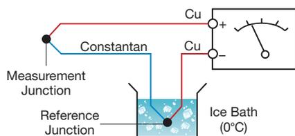
▲ **Figure 2.** The reference junction of a standard thermocouple is held constant. This reference junction is held at 0°C.
