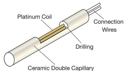
▲ **Figure 6.** In one type of RTD, platinum wires are wound around a mandrel and encased in ceramic.
