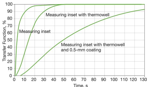
▲ **Figure 7.** Thermocouples and RTDs installed in thermowells have longer response times than bare sensors. Coated thermowells have even longer response times.
