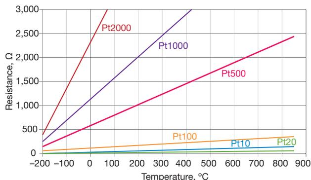
▲ **Figure 5.** The resistance of an RTD increases with temperature and is a function of the metal.
