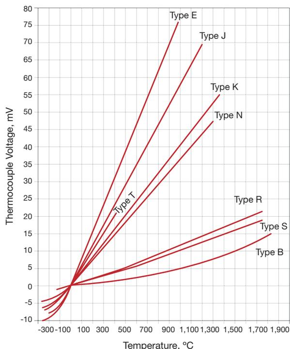
▲ **Figure 3.** Each type of thermocouple has unique thermal voltage characteristics. The voltage response is a function of temperature.
